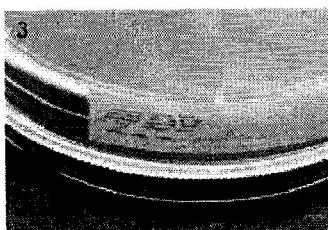
3 Lid with yellow inscription field as well as spacers on the inside of the lid.
